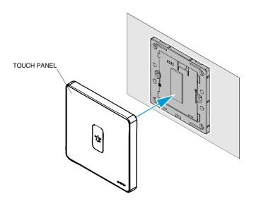
4. Carefully press the touch panel by applying even force on all sides until it is seated securely on the switch module.
